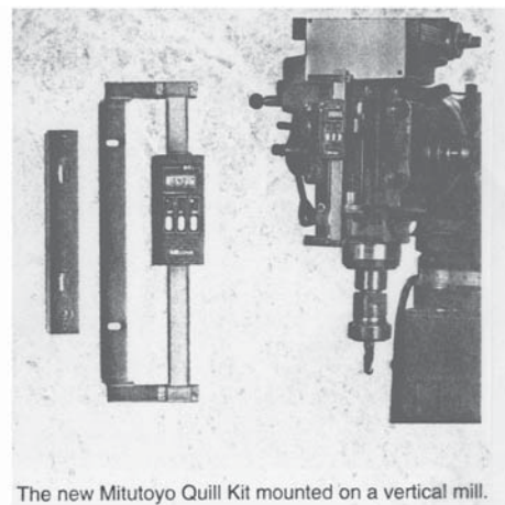
The new Mitutoyo Quill Kit mounted on a vertical mill.
